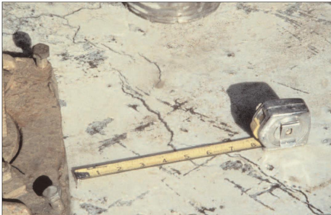
**FIGURE 8.3.** Plastic shrinkage cracks in silica-fume concrete.
