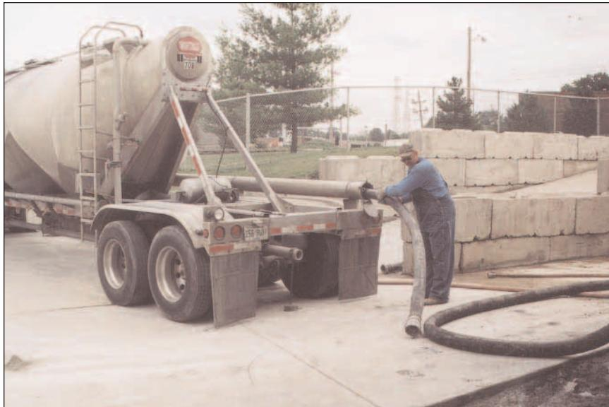
**FIGURE 7.5A.** Rubber hose used to transfer silica fume from tanker to producer's silo.
